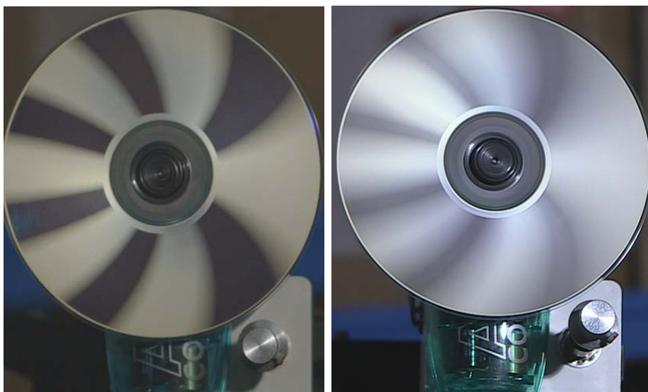
Figure 14, Rolling shutter effect, a) 1/1000 b) 1/50
